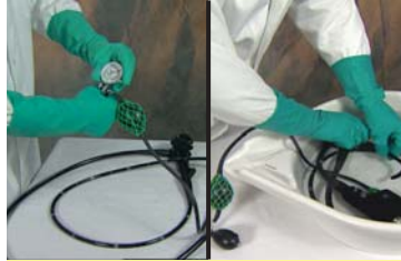
STAGE 1/Dry Test STAGE 2/Wet Test
