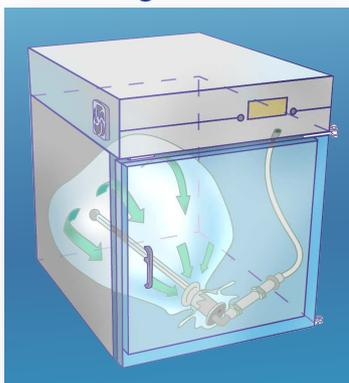
The Anprolene and EOGas Series 4 sterilisers use a purge probe. The sterilisation bag is sealed around the bobbin on the purge probe.
