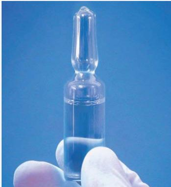
The Andersen system supplies the EtO for sterilisation in a glass ampoule. In the Anprolene refill kits the glass ampoule is held within a break shield. In the EOGas refill kits the ampoule is held within a plastic cartridge.
