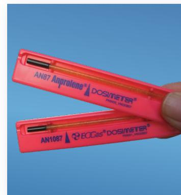
A unique chemical integrator has been developed by Andersen Products, with specific versions for use at room temperature and at 50°C. These integrate the effects of EtO gas concentration, temperature and exposure duration. A colour change from orange to blue proceeds up the tube (from left to right) and signals a successful cycle when it passes the blue triangle on the pink backing plate.
